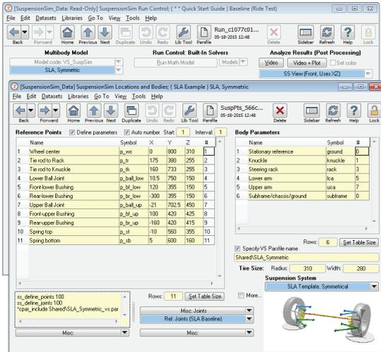
Model users can make variant suspensions using only a few screens.
