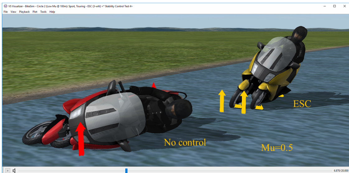
Figure 11. TWS models with and without stability control at 145 km/h speed on a constant radius of curve and road friction of 0.5.
