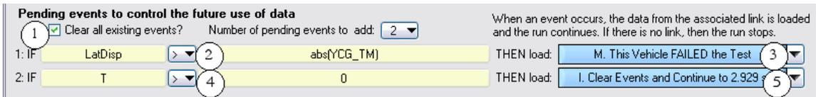
Figure 24. New pending events added by Events dataset H to check lateral displacement.
